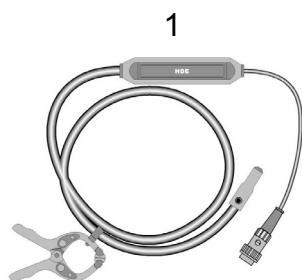
Hall-effect rpm sensing
